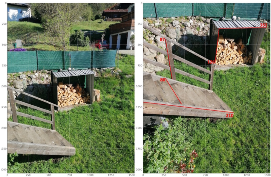
Fig. 3. Results from Object Measurement Based on Triangulation (in cm)
